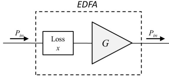
Without the loss section (that is when  $x = 1$ ) the EDFA has a noise figure of  $NF = 2n_{sp} = 5$  dB. When installed the loss is actually of 3 dB ( $x = 0.5$ ). We want to calculate the noise figure of the lossy amplifier (the relation  $NF = 2n_{sp}$  does not hold anymore).
